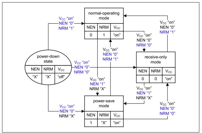
Figure 5 Power-up and undervoltage
