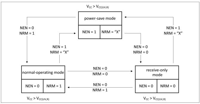
Figure 4 Mode state diagram
