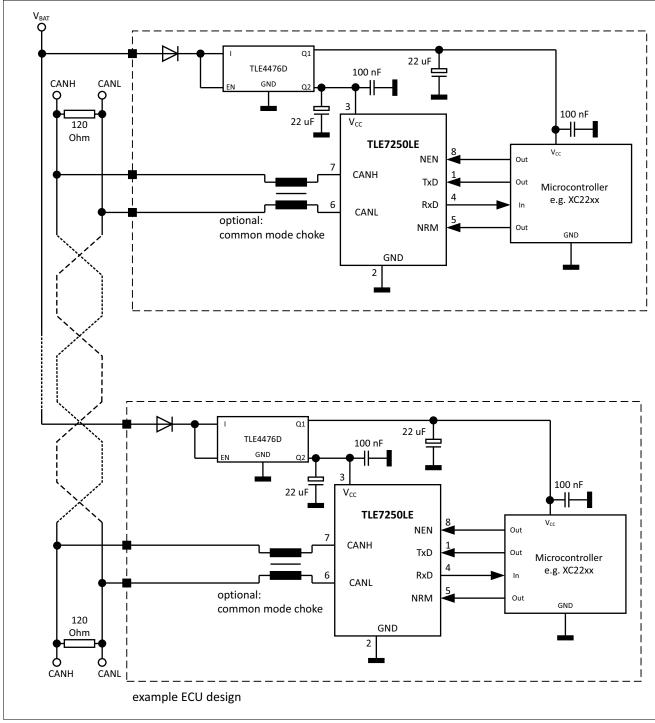
Figure 12 Application circuit
