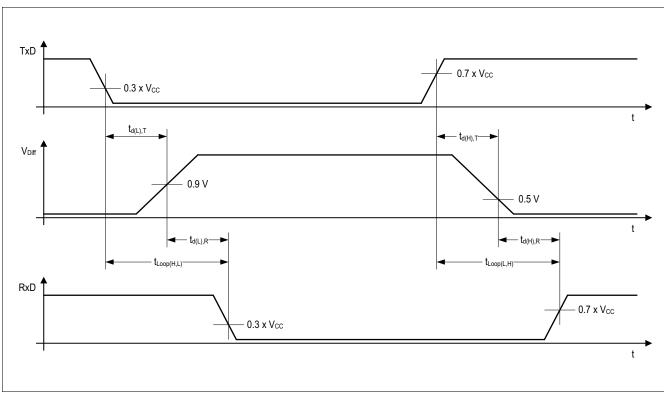
Figure 10 Timing diagrams for dynamic characteristics
