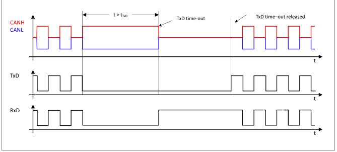
Figure 7 TxD time-out function
