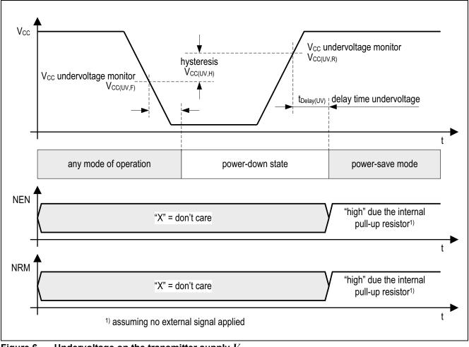
Figure 6 Undervoltage on the transmitter supply  $V_{\rm CC}$
