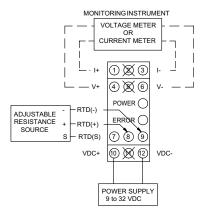
**Field Calibration Wiring**
