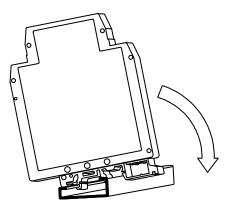
To install the IRMA on a "T" style rail, angle the module so that the top groove of the "foot" is located over the lip of the top rail. Push the module toward the rail until it snaps into place. To remove a module from the rail, insert a screwdriver into the slot on the bottom of the "foot", and pry upwards on the module until it releases from the rail.
