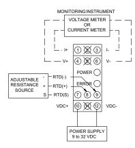
Basic Calibration Wiring
