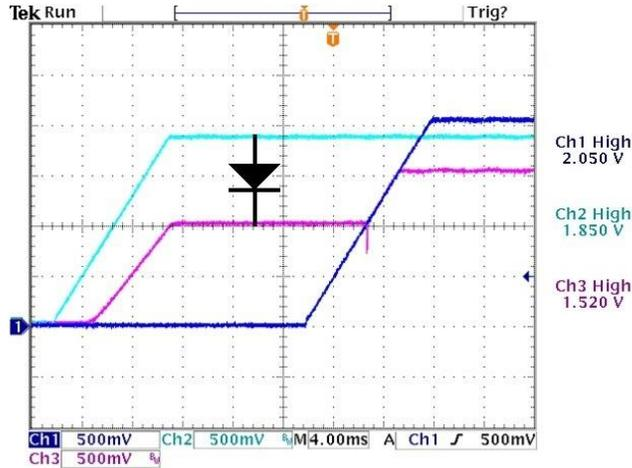
Figure 20 was captured with an actual system where a diode was added to pre-bias a 1.5V bus from a 1.85V bus in order to simulate the effect of current leakage through protection circuits of unpowered logic connected to powered logic outputs (a common source of pre-bias in power systems).
