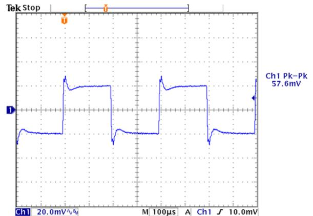
As the Load Regulation parameter is increased, step offsets in output voltage begin to appear, as shown in Figure 9. The Load Regulation parameter is an important part of Current Sharing. It is used to set one dPOL as a "master", by assigning a lower mV/A load regulation than all other dPOLs which share the load as "slaves". The dPOL with the lowest Regulation parameter sets the effective overall regulation. (See Current Sharing elsewhere in this document.)
