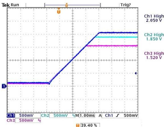
Figure 17. Turn-On with Slew Rates Programmed as follows: V1 at 1.0V/ms, V2 at 0.5V/ms, V3 at 0.2V/ms. Vin=12V
