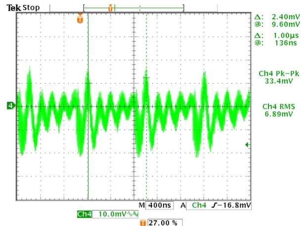
Figure 39 shows the input voltage noise of the three-output system with programmed interleave. Instead of all three dPOLs switching at the same time as in the previous example, the dPOLs V1, V2, and V3 switch at 67.5°, 180°, and 315°, respectively. Noise is spread evenly across the switching cycle resulting in more than 1.5 times reduction. To achieve similar noise reduction without the interleave will require the addition of an external LC filter.
