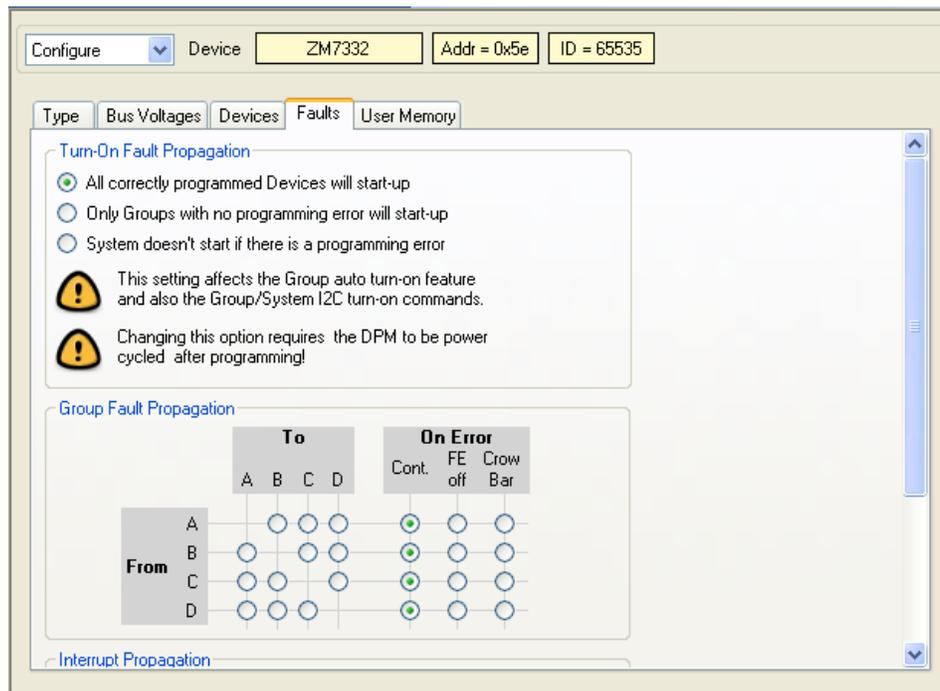
Note that the turn-off type of the fault as it propagates through the DPM will remain unchanged. Propagation options for dPOLs can be read or set in the dPOL PC3 register shown in Figure 30.
