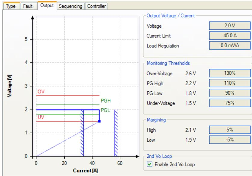
Note that the GUI shows the effect of setting PG, OV and UV limits as both values and graphical limit bars. Vertical hashed lines are error bars for the Overcurrent (OC) limit.
