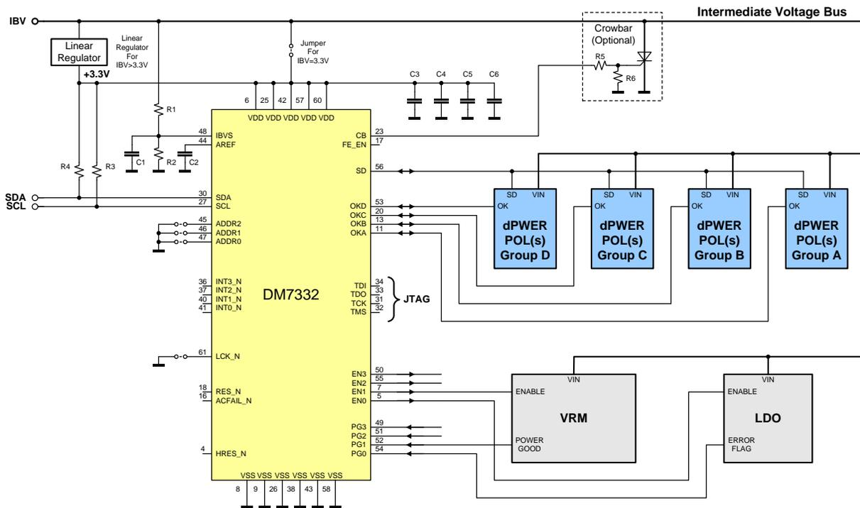
Shown in Figure 50 is a schematic of a typical application using at least one DP7160G dPOL. Although additional DP7160G or other d-pwer® series dPOLs (Note SD and OK dashed lines "TO OTHER dPOLs") may be connected.
