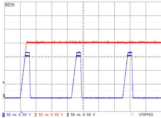
Since both Vo1 and Vo2 have the same delay and slew rate settings they will continue to turn off and on synchronously every 130ms as shown in Figure 34 until the condition causing the undervoltage is removed.
