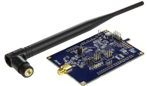
The 868MHz monopole antenna is connected to the SMA connector of the PCB and the external power supply or battery has to be connected to connector X1.
