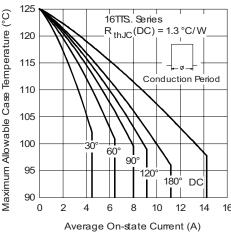
Fig. 2 - Current Rating Characteristics
