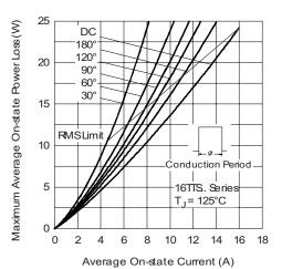
Fig. 4 - On-State Power Loss Characteristics
