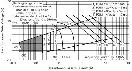
Fig. 9 - Gate Characteristics
