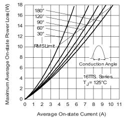
Fig. 3 - On-State Power Loss Characteristics
