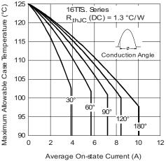
Fig. 1 - Current Rating Characteristics
