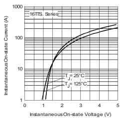
Fig. 7 - On-State Voltage Drop Characteristics
