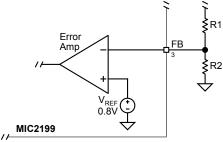
Figure 6. Voltage-Divider Configuration
