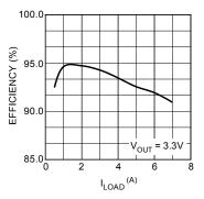
Efficiency for V<sub>IN</sub> = 5V and V<sub>OUT</sub> = 3.3V
