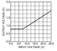
Figure 5. Minimum Output Voltage vs. Input Supply Voltage
