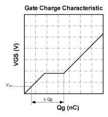
Figure 9. MOSFET Gate Charge Characteristic
