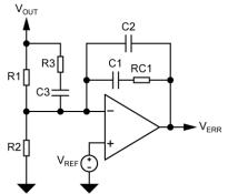
Figure 14. Type II Compensation Network
