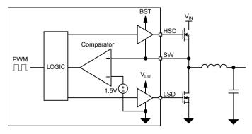
Figure 8. Adaptive Gate Drive Diagram
