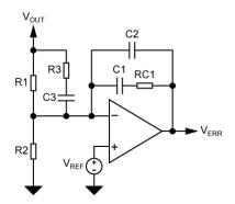
Figure 12. Type III Compensation Network
