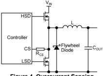
Figure 4. Overcurrent Sensing
