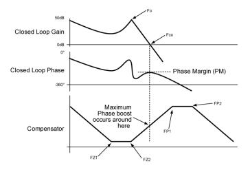
Figure 11. Ceramic Output Capacitor Bode Plot
