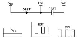
Figure 7. High-Side Gate Drive Circuit and Waveform
