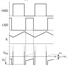
Figure 5. Current Sensing Waveforms
