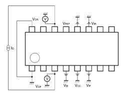
VcE is the sum of the high- and low-side output transistor C-E voltages. The direction of the Io current is from the HIGH level to the LOW level output pin.
