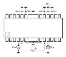
VcE is the sum of the high- and low-side output transistor C-E voltages. The direction of the lo current is from the HIGH level to the LOW level output pin.
