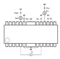
Refer to the truth table for output mode. The supply current is represented by the Icc-value, and the VREF sink current is represented by the IREF-value. The direction of the Ic current is from the HIGH level to the LOW level output pin.
