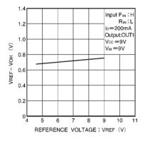
Fig.18 VREF-VoH voltage vs. VREF reference voltage
