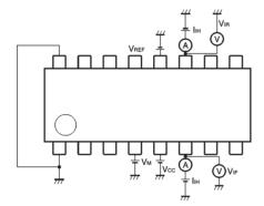
\* Refer to the truth table for output mode. HIGH and LOW level input voltages correspond to the readings of V IF and VIR voltmeters, respectively. The HIGH level input current is represented by the IIH ammeter reading when VIN = 2 V.
