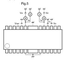
\* Refer to the truth table for output mode. HIGH and LOW level input voltages correspond to the readings of  $V_{\rm IR}$  and  $V_{\rm IR}$  voltmeters, respectively. The HIGH level input current is represented by the IIH ammeter reading when  $V_{\rm IN} = 2 \ V$ .
