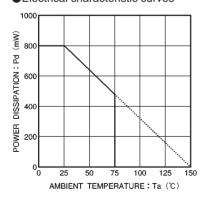
Fig.12 Temperature dependence of power dissipation curve (BA6285FS)
