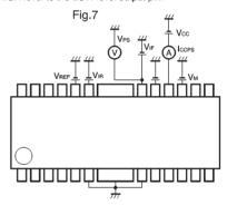
The power save mode ON voltage is represented by the VPs reading when IccPs is  $15~\mu\mathrm{A}$  or less. The power save mode OFF voltage is represented by the VPs reading when IccPs is more than  $15~\mu\mathrm{A}$ .
