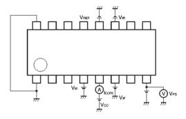
The power save mode ON voltage is represented by the VPs reading when lccps is 15  $\mu$ A or less. The power save mode OFF voltage is represented by the VPs reading when lccps is more than 15  $\mu$ A.
