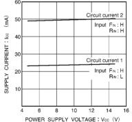
Fig.14 Supply current vs. power supply voltage
