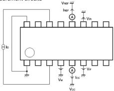
Refer to the truth table for output mode. The supply current is represented by the Icc-value, and the Vret sink current is represented by the IREF-value. The direction of the Io current is from the HIGH level to the LOW level output pin.
