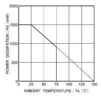
Fig.13 Temperature dependence of power dissipation curve (BA6285FP)
