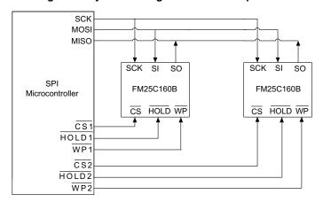
Figure 2. System Configuration with SPI port
