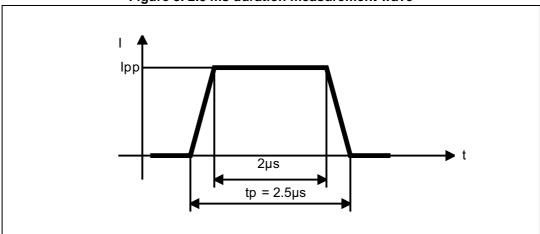
Figure 3. 2.5 ms duration measurement wave
