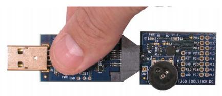
Figure 2. Improper Method of Holding the ToolStick
