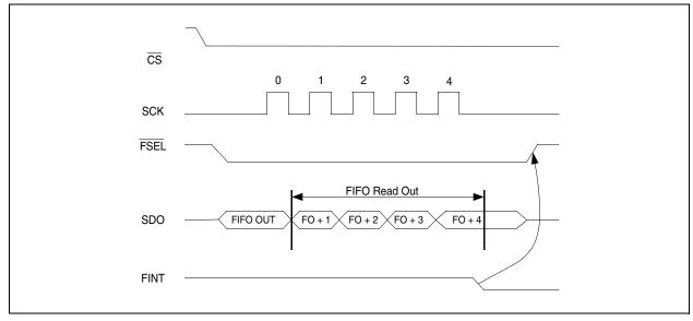
**Note:** During FIFO access, fsck cannot be higher than fref/4, where fref is the crystal oscillator frequency. If the duty cycle of the clock signal is not 50%, the shorter period of the clock pulse should be at least 2/fref.
