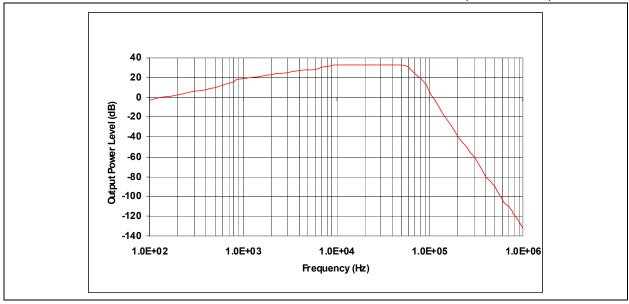
The receive bandwidth is programmable from 67 kHz to 400 kHz to accommodate various FSK modulation deviations. If the deviation is known for a given transmitter, good results are obtained with a bandwidth of at least twice the transmitter FSK deviation.
