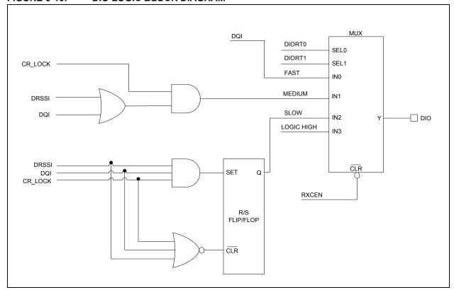
The DIO signal response time setting is configured through RXCREG and has the following modes of operation:
