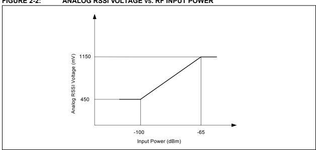
FIGURE 2-2: ANALOG RSSI VOLTAGE vs. RF INPUT POWER
