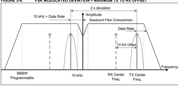
FIGURE 3-9: **FSK MODULATED DEVIATION – MAXIMUM TX TO RX OFFSET**
