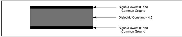
FIGURE 4-4: FOUR BASIC COPPER FR4 LAYERS
