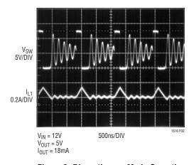
Figure 2. Discontinuous Mode Operation
