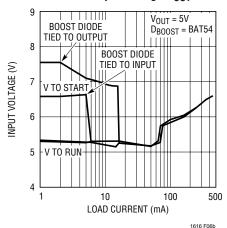
Figure 6. The Minimum Input Voltage Depends on Output Voltage, Load Current and Boost Circuit
