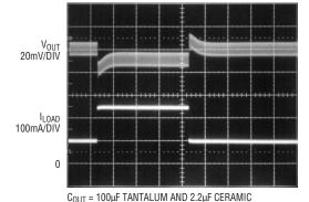
Figure 3. Transient Load Response of the LT1616
