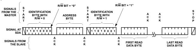
FIGURE 9. MULTIPLE BYTES READ SEQUENCE
