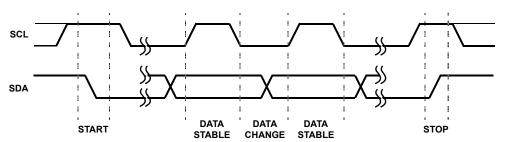
FIGURE 5. VALID DATA CHANGES, START, AND STOP CONDITIONS
