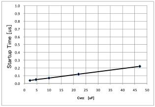
Figure 6. Startup Time (Reference Value) (C<sub>VCC</sub> is capacitance for the VCC pin.)
