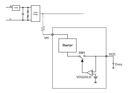
Figure 4. Block Diagram of Start Circuit
