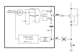
Figure 23. CS Pin Peripheral Circuit
