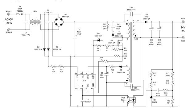
Figure 28. Application Circuit Example
