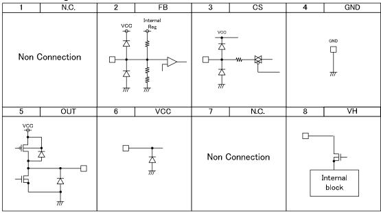
Figure 2. I/O Equivalent Circuit Diagram
