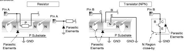
Figure 31. Example of monolithic IC structure
