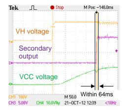
Figure 9. Waveform of No-load Startup
