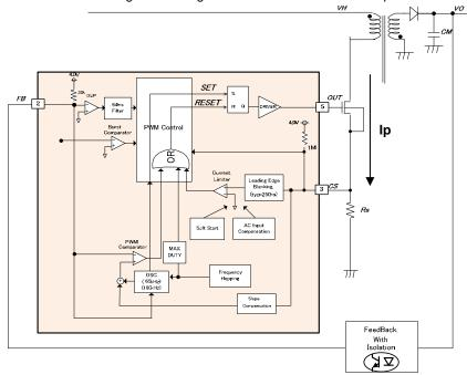
Figure 13. Block Diagram of IC Internal PWM Operations
