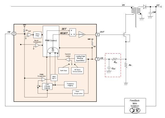
Figure 22. Circuits Peripheral to the CS Pin
