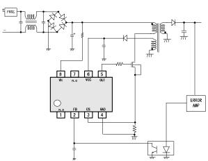
Figure 1. Application Circuit
