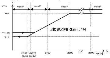
Figure 18 FB Voltage and CS Voltage Characteristics
