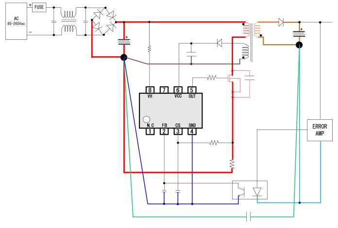
Figure 27. Board Layout Pattern
