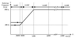
Figure 17. Operation with FB pin voltage
