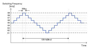
Figure 16. Frequency Hopping Function
