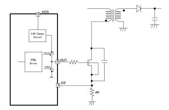
Figure 25. OUT Pin (Pin 5) Schematic
