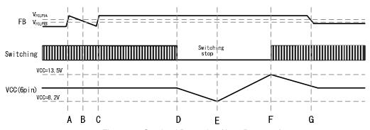
Figure 24. Overload Protection (Auto Recovery)
