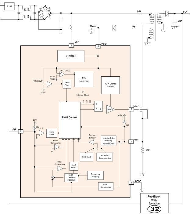
Figure 3. Block Diagram
