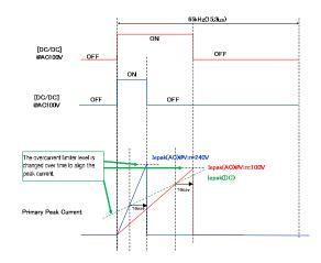
Figure 19. Without AC Voltage Compensation Function
