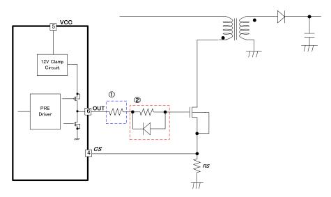
Figure 26. OUT Pin (Pin 5) Driver Circuit
