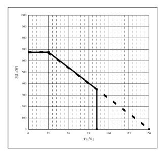
Figure 30. Thermal Abatement Characteristics
