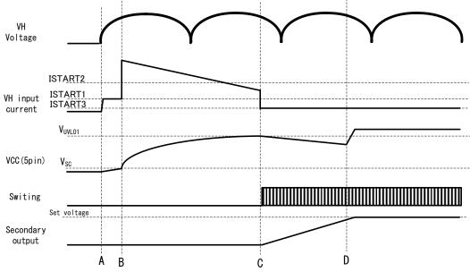
Figure 7. Operating Waveform at Startup
