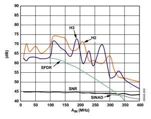
Figure 9. Analog Input Frequency Sweep,  $A_{IN} = -1 \text{ dBFS}$ , FS = 0.75 V, fs = 250 MSPS, External VREF Mode
