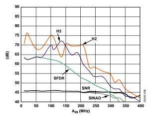
Figure 8. Analog Input Frequency Sweep,  $A_{IN} = -1 \text{ dBFS}, \text{ FS} = 1 \text{ V}, \text{ fs} = 250 \text{ MSPS}$
