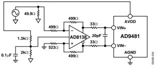
Figure 29. Driving the ADC with the AD8138
