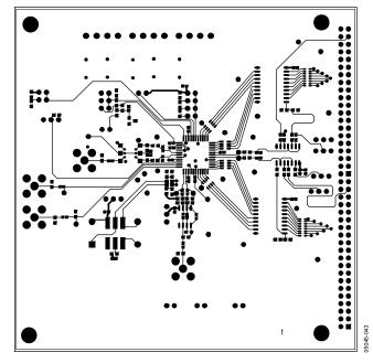
Figure 42. PCB Top-Side Copper Routing
