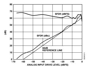
Figure 11. SFDR vs. A<sub>IN</sub> Input Level; A<sub>IN</sub> = 70 MHz @ 250 MSPS
