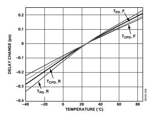
Figure 22. Propagation Delay Sensitivity vs. Temperature
