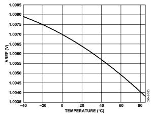
Figure 32. Typical Reference Variation with Temperature
