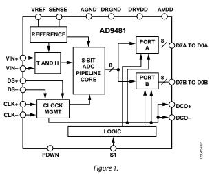
The AD9481 is available in a Pb-free, 44-lead, surface-mount package (TQFP-44) specified over the industrial temperature range ( $-40^{\circ}$ C to  $+85^{\circ}$ C).
