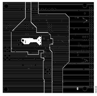
Figure 44. PCB Split Power Plane
