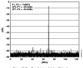
Figure 12. Two-Tone Intermodulation Distortion (69.3 MHz and 70.3 MHz; f<sub>s</sub> = 250 MSPS)
