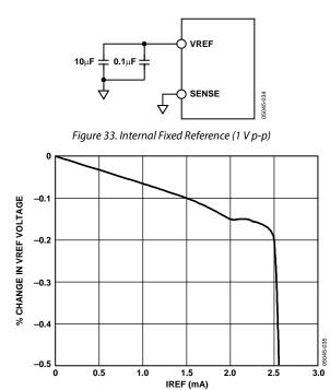
Figure 34. Internal VREF vs. Load Current
