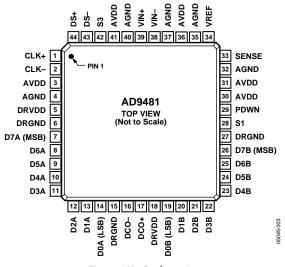
Figure 3. Pin Configuration
