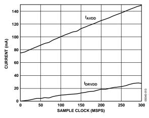
Figure 13.  $I_{AVDD}$  and  $I_{DRVDD}$  vs. Clock Rate,  $C_{LOAD} = 5 \text{ pF}$  $A_{IN} = 70 \text{ MHz} @ -1 \text{ dBFS}$
