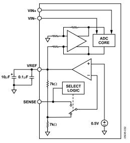
Figure 31. Internal Reference Equivalent Circuit
