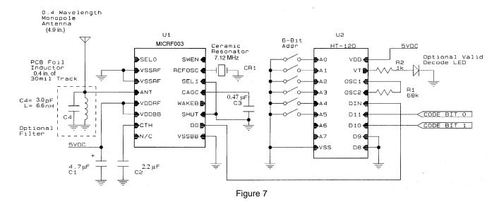
915MHz, 1kbps OOK Receiver/Decoder SWP Mode, Continuous Operation 6-Bit Address Decode/2 OP Codes
