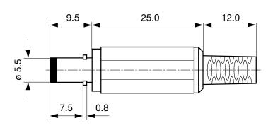
Cable diameter max. 4.0 mm
