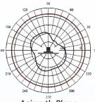
Azimuth Plane Cut perpendicular to the antenna, parallel to the connector/cable exit, perpendicular to the polarization
