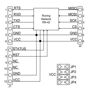
Figure 1. PmodBT2 block diagram.
