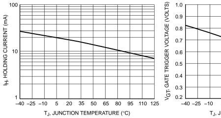
Figure 5. Typical Holding Current versus Junction Temperature
