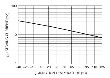
Figure 7. Typical Latching Current versus Junction Temperature
