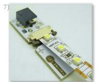
Make sure the LED strip is centered and fully inserted into the LED connector. You may need to hold the latch open with one hand so that the adhesive doesn't pull the latch closed prematurely.
