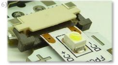
Insert the flexible LED strip into the **open** LED connector: above the sliding latch and below the beige top. Again, make sure that the positive side of the strip matches the positive side of the board.
