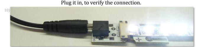
If there is any flickering, make sure flex is fully inserted and that the latch is secure. If no lights turn on, check polarity.
