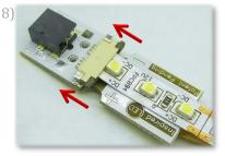
Secure the LED connector by closing the sliding latch. Again, the adhesive may want to resist. Your thumb nails are your friend here.
