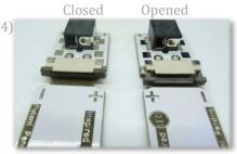
Also notice the LED connector - it opens for easy strip insertion and latches to secure the connection.
