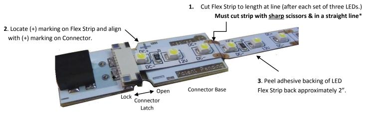
**4**. Holding latch open with thumb and forefinger slide Flex Strip fully into connector, slide latch to full lock position and press Flex Strip onto Connector Base.
