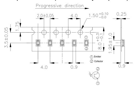
Note: The tolerances unless mentioned are ±0.1mm, Unit: mm
