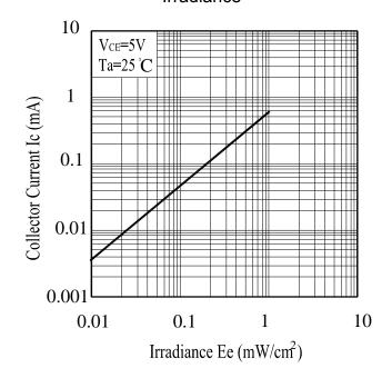
Fig.3 Collector Current vs.
