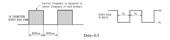
Fig.-2 Measuring Method
