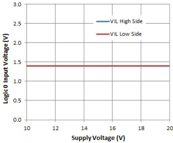
Figure 22. Logic 0 Input Voltage vs. Supply Voltage
