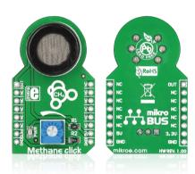
Methane click<sup>™</sup> is a simple solution for adding a high sensitivity methane (CH<sub>4</sub>) sensor to your design. It's suitable for designing gas leakage equipment. The board features an MQ-4 sensor, a calibration potentiometer, a mikroBUS<sup>™</sup> host socket, two jumpers and a power indicator LED. Methane click<sup>™</sup> communicates with the target board through mikroBUS<sup>™</sup> AN (OUT) line. Methane click<sup>™</sup> is designed to use a 5V power supply only.
