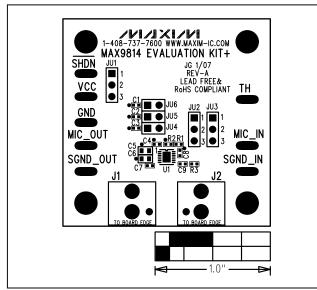
Figure 2. MAX9814 EV Kit Component Placement Guide— Component Side
