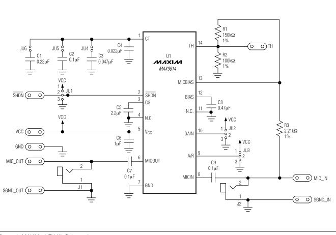
Figure 1. MAX9814 EV Kit Schematic
