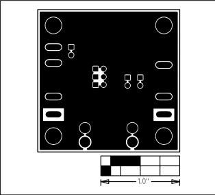
Figure 4. MAX9814 EV Kit PCB—Solder Side
