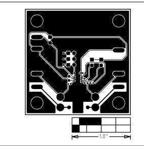
Figure 3. MAX9814 EV Kit PCB—Component Guide
