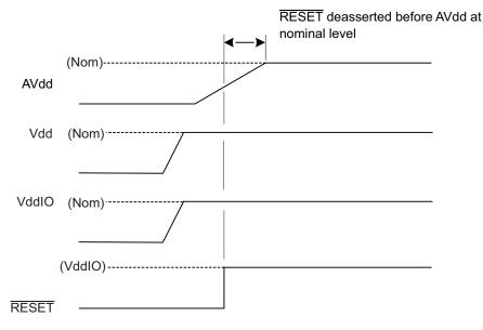
The RESET pin can be used to reset the device whenever necessary. The RESET pin must be asserted low for at least 90 ns to cause a reset. After releasing the RESET pin the device typically takes 90 ms before it is ready to start communications. It is recommended to connect the RESET pin to a host controller to allow it to initiate a full hardware reset without requiring a power-down.
