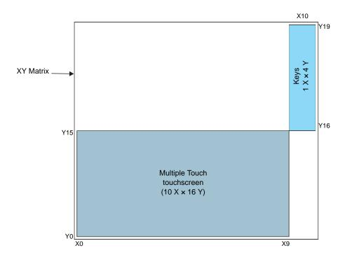
If, however, the intention is to preserve a larger touchscreen size and maintain an optimal aspect ratio, then using equal X and Y lines for the key array can be considered, as in Figure 4-2.
