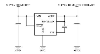
An LDO regulator should be chosen that provides adequate output capability, low noise, good load regulation and step response. The voltage regulators listed in Table 10-1 have been tested and found to work well with maXTouch devices. If it is desired to use an alternative LDO, however, certain performance criteria should be verified before using the device. These are:
