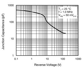
Fig. 5 - Typical Junction Capacitance
