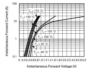
Fig. 3 - Typical Instantaneous Forward Characteristics
