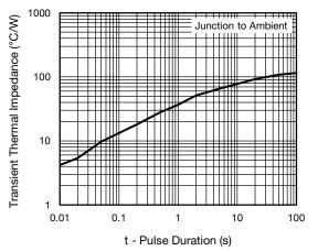
Fig. 6 - Typical Transient Thermal Impedance
