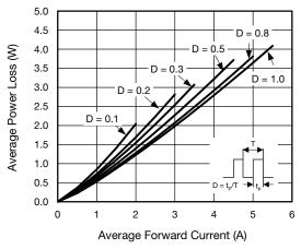
Fig. 2 - Forward Power Loss Characteristics
