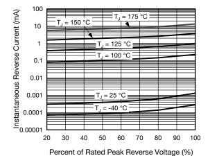
Fig. 4 - Typical Reverse Leakage Characteristics
