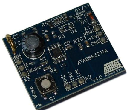
Figure 1. Atmel ATAB663211A Development Board
