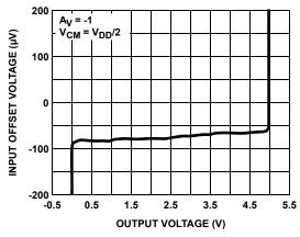
FIGURE 4. INPUT OFFSET VOLTAGE vs OUTPUT VOLTAGE
