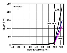
FIGURE 18.  $I_{BIAS+}$  vs TEMPERATURE,  $V_S = \pm 2.5V$
