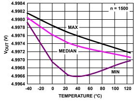
FIGURE 25.  $V_{OUT}$  HIGH vs TEMPERATURE,  $V_{S}$  = ±2.5V,  $R_{L}$  = 100k
