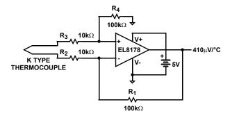
FIGURE 30. THERMOCOUPLE AMPLIFIER
