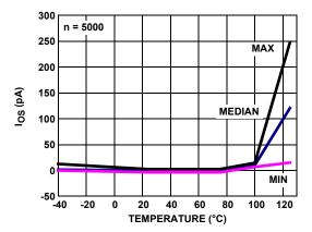
FIGURE 20.  $I_{OS}$  vs TEMPERATURE,  $V_S = \pm 2.5 V$
