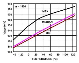
FIGURE 26.  $V_{OUT}$  LOW vs TEMPERATURE,  $V_{S}$  = ±2.5V,  $R_{L}$  = 1k
