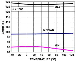
FIGURE 22. CMRR vs TEMPERATURE, V+ = ±2.5V, ±1.5V
