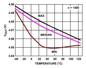
FIGURE 24.  $V_{OUT}$  HIGH vs TEMPERATURE,  $V_{S}$  = ±2.5V,  $R_{L}$  = 1k
