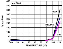
FIGURE 19.  $I_{BIAS}$  vs TEMPERATURE,  $V_S = \pm 2.5V$
