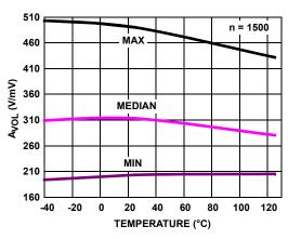
FIGURE 21. A $_{VOL}$  vs TEMPERATURE, R $_{L}$  = 100k, V $_{O}$  = ±2V @ V $_{S}$  = ±2.5V
