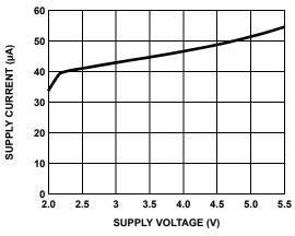
FIGURE 3. SUPPLY CURRENT vs SUPPLY VOLTAGE
