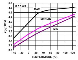
FIGURE 27.  $V_{OUT}$  LOW vs TEMPERATURE,  $V_{S}$  = ±2.5V,  $R_{L}$  = 100k
