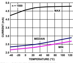
FIGURE 15. DISABLED SUPPLY CURRENT vs TEMPERATURE, V<sub>S</sub> = ±2.5V
