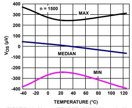
FIGURE 16.  $V_{OS}$  vs TEMPERATURE,  $V_{S}$  = ±2.5V
