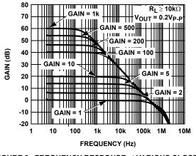
FIGURE 2. FREQUENCY RESPONSE at VARIOUS CLOSED LOOP GAINS
