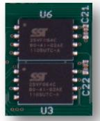
The serial FLASH devices are connected to the **RSPI0** port of the RX MCU:
