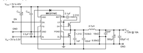
Synchronous Buck Controller Featuring Adaptive On-Time Control
