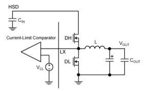
Figure 4. MIC2174/MIC2174C Current Limiting Circuit
