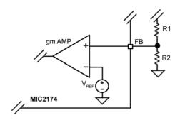
Figure 8. Voltage-Divider Configuration
