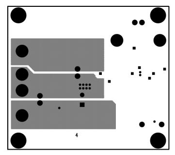
Figure 12. MIC2174/MIC2174C Evaluation Board Bottom Layer
