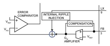
Figure 9. Internal Ripple Injection
