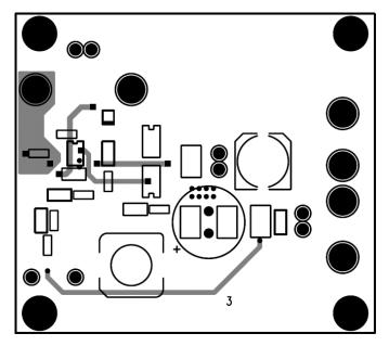
Figure 14. MIC2174/MIC2174C Evaluation Board Mid-Layer 2
