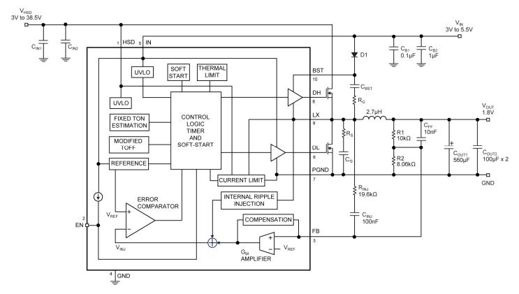
Figure 1. MIC2174/MIC2174C Block Diagram
