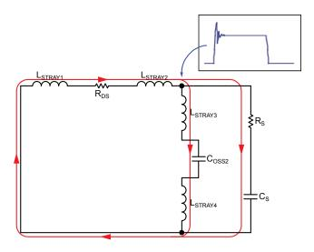
Figure 6. Snubber Circuit
