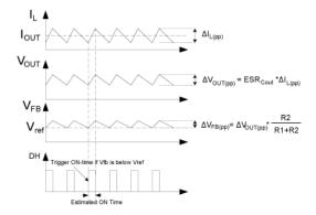
Figure 2. MIC2174/MIC2174C Control Loop Timing
