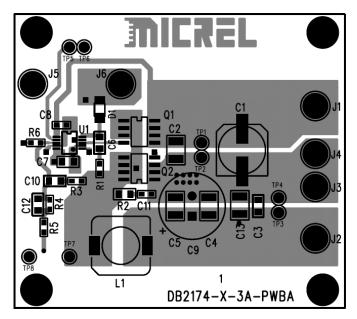
Figure 11. MIC2174/MIC2174C Evaluation Board Top Layer
