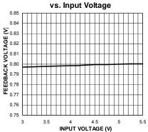
Feedback Voltage vs. HSD Voltage
