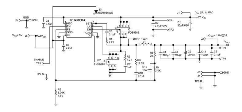
Figure 10. Schematic of MIC2174/MIC2174C Evaluation Board
