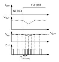
Figure 3. MIC2174/MIC2174C Load-Transient Response
