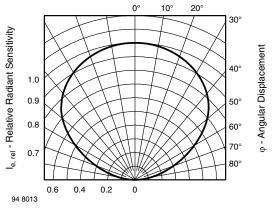
Fig. 2 - Radiant Characteristics  $I_{rel} = f(\phi)$
