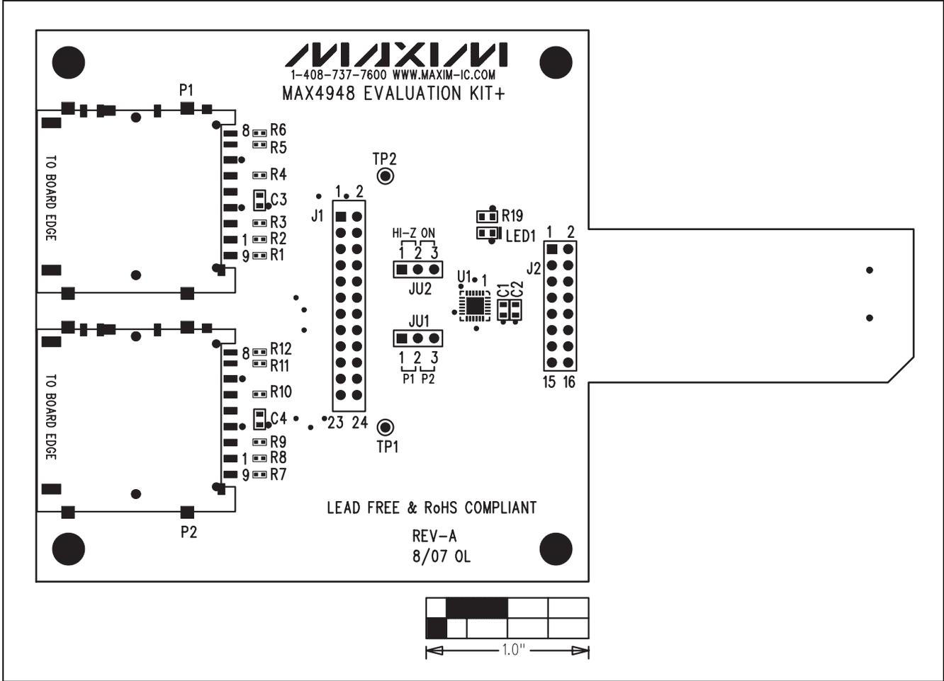
Figure 5. MAX4948 EV Kit Component Placement Guide—Component Side
