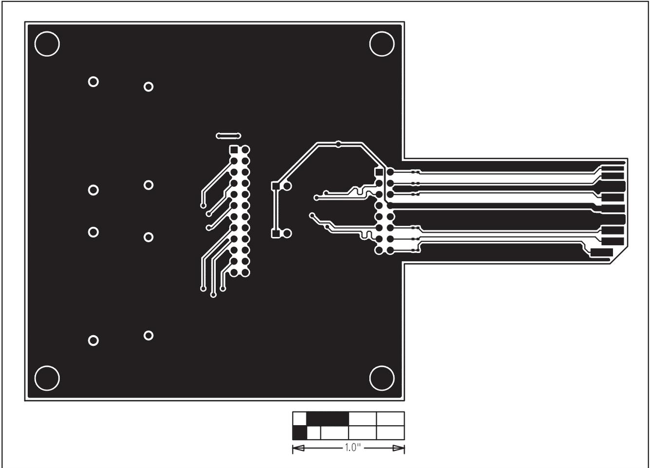
Figure 7. MAX4948 EV Kit PCB Layout—Solder Side
