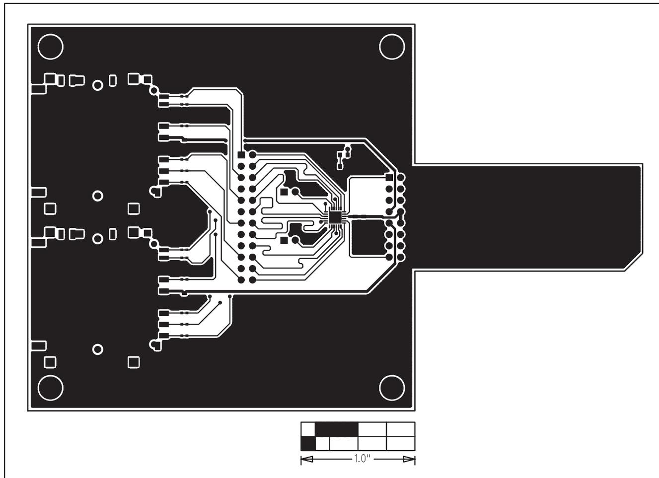
Figure 6. MAX4948 EV Kit PCB Layout—Component Side
