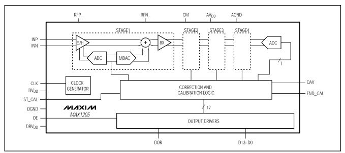
Figure 1. Internal Block Diagram
