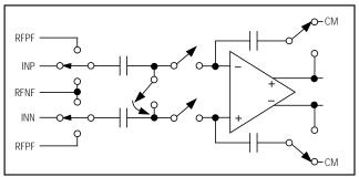
Figure 2. Simplified MDAC Architecture
