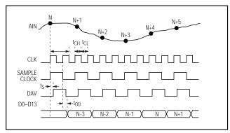
Figure 7. Main Timing Diagram
