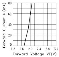
Fig.2 FORWARD CURRENT VS. FORWARD VOLTAGE
