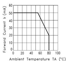
Fig. 3 FORWARD CURRENT DERATING CURVE
