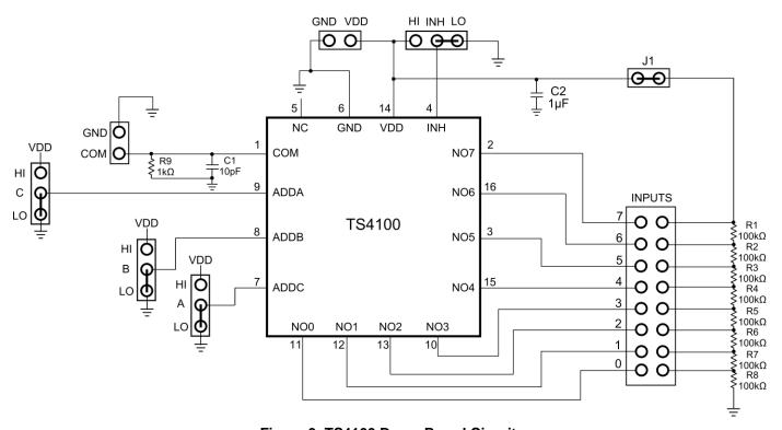
Figure 3. TS4100 Demo Board Circuit
