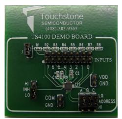
Figure 1. TS4100 Demo Board (Top View)
