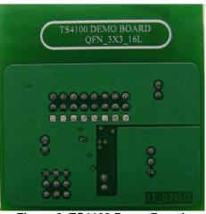
Figure 2. TS4100 Demo Board (Bottom View)
