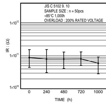
Fig.24 Insulation resistance
