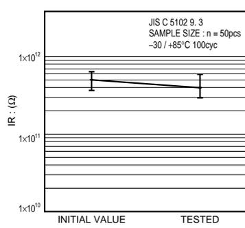
Fig.15 Insulation resistance
