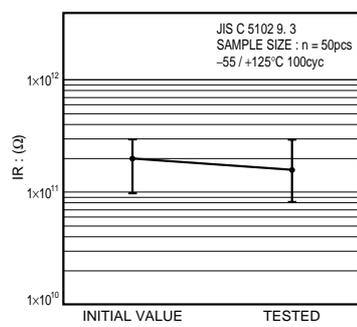
Fig.12 Insulation resistance
