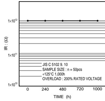
Fig.18 Insulation resistance
