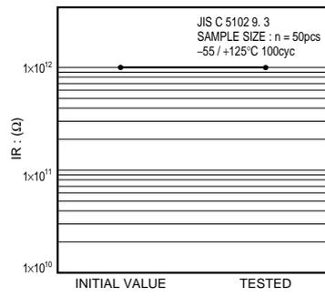
Fig.9 Insulation resistance
