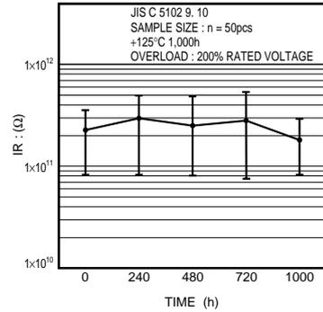
Fig.21 Insulation resistance
