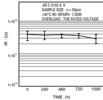
Fig.30 Insulation resistance
