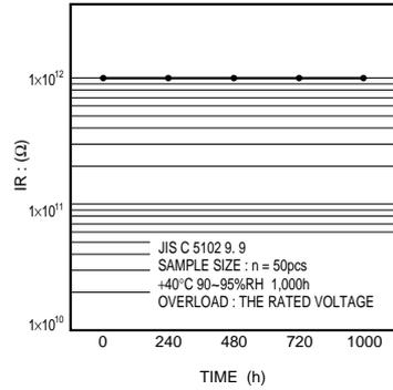
Fig.27 Insulation resistance
