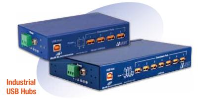
Our  $Ulinx^{\text{TM}}$  industrial USB hubs are designed with rugged metal cases, versatile mounting options, high ESD protection, wide operating temperature ranges and high retention USB connectors for instant plug-and-play connectivity.
