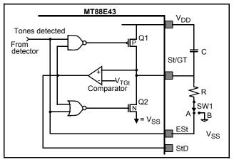
Figure 4 - Guard Time Circuit Operation
