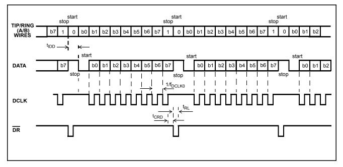
Figure 14 - Serial Data Interface Timing (MODE 0)
