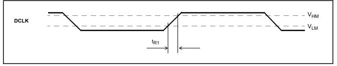
Figure 15 - DCLK Mode 1 Input Timing
