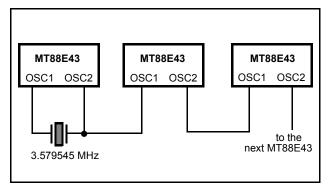
Figure 8 - Common Crystal Connection
