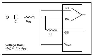
Figure 6 - Single-Ended Input Configuration
