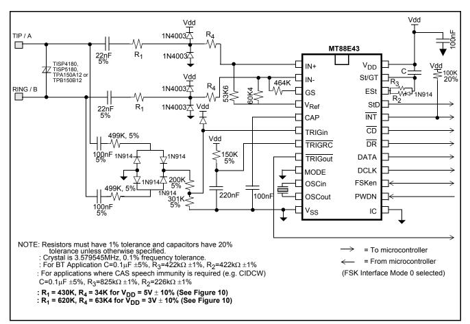
Figure 9 - Application Circuit
