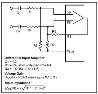
Figure 7 - Differential Input Configuration
