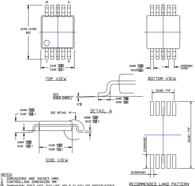
1. DIMENSIONS ARE INCHES LMMIJ. 2. CONTROLLING DIMENSION: MM 3. DIMENSION DOES NOT INCLUDE MOLD FLASH OR PROTRUSIONS, EITHER OF WHICH SHALL NOT EXCEED 0.008 [0.20] PER SIDE. 10-Pin MSOP (MM)
