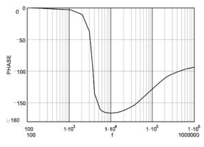
Figure 6. The Phase Curve with ESR =  $0.002\Omega$
