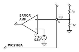
Figure 2. Voltage-Divider Configuration
