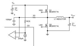
Figure 1. MIC2168A Current Limiting Circuit
