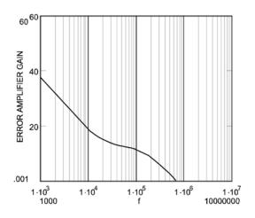
Figure 7. Error Amplifier Gain Curve
