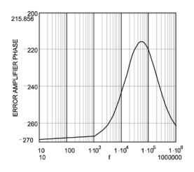
Figure 8. Error Amplifier Phase Curve
