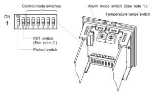
Note: 1. The alarm mode switch is not provided on models without an alarm.
