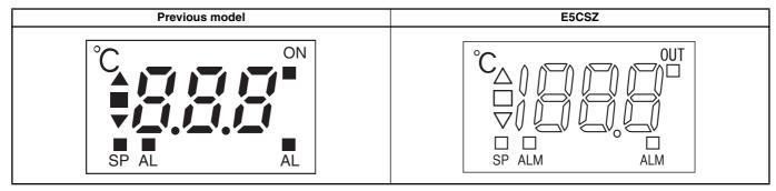
The display digits can be increased up to 1,999. The display "ON" has changed to "OUT" and "AL" has changed to "ALM."
