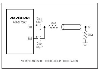
Figure 1. Output with SAG Correction
