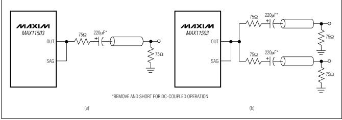
Figure 2. Traditional AC-Coupled Output
