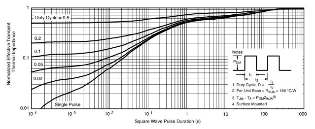
Normalized Thermal Transient Impedance, Junction-to-Ambient
