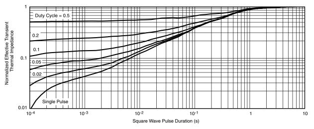
Normalized Thermal Transient Impedance, Junction-to-Foot
