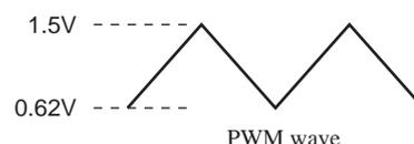
$$PWMduty = \frac{V_{OUT}}{V_{IN} - V_{sat} + VF} = 23 \%$$
