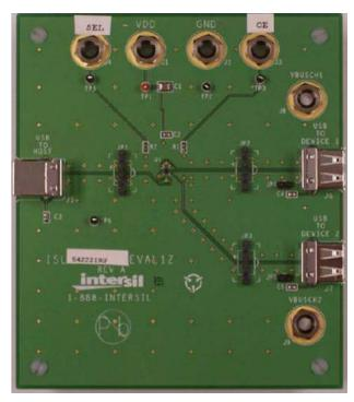
FIGURE 1. ISL54222AIRUEVAL1Z EVALUATION BOARD
