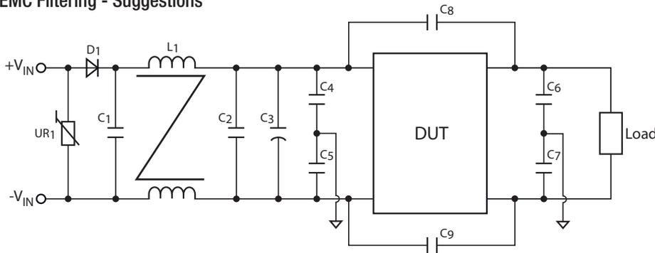
It is recommended to add UR1 and D1 in railway application. C1, C2, C3 & L1 can be modified for required EMI standards. To meet EN61000-4-2, module case should be earth grounded. We offer independent case pin option on request, the location is between pin 2 and pin 6.
