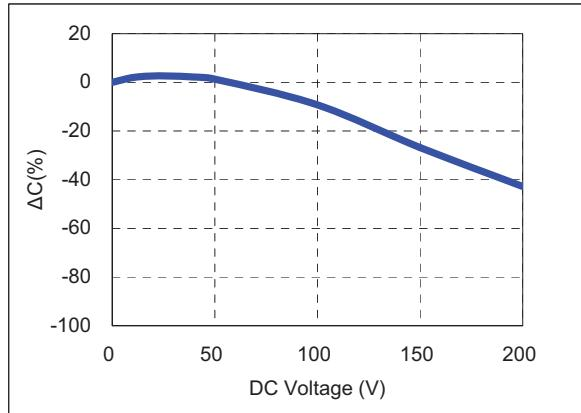
4) Bias TCC characteristics (Agilent 4284A, 1kHz, 1Vrms, 100Vdc)
