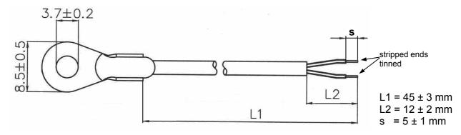
dimensions in mm, tolerances unless specified acc. to DIN ISO 2768-m
